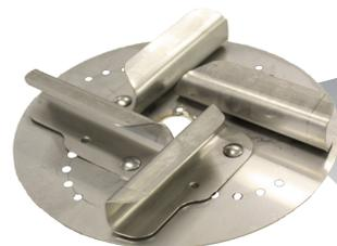
When looking down at the spinner, moving the fins counter-clockwise will adjust the spread pattern toward the right side of the spreader.
