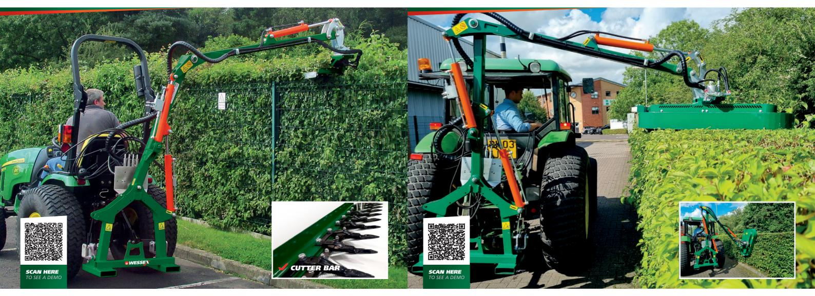
The Wessex **CHT-120** 1.2m hedge cutter is perfect for trimming small trees, hedges and pruning edges, and are ideal for compact tractors of 15hp and above. The model features a 1.2m cutter bar and comes complete with hydraulic spool lever controls. Note\* electric joystick controls required for enclosed
